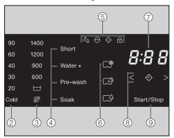
The ②, ③, ④, ⑥, ⑧ and ⑨ sensors react to fingertip contact. Selection is possible as long as the respective sensor is illuminated.
