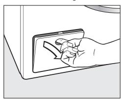
Open the drain pump access panel.
