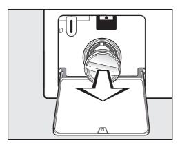
Remove the drain filter completely.
